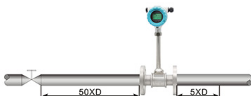
Regulating Valve, Half-open Gate Valve
