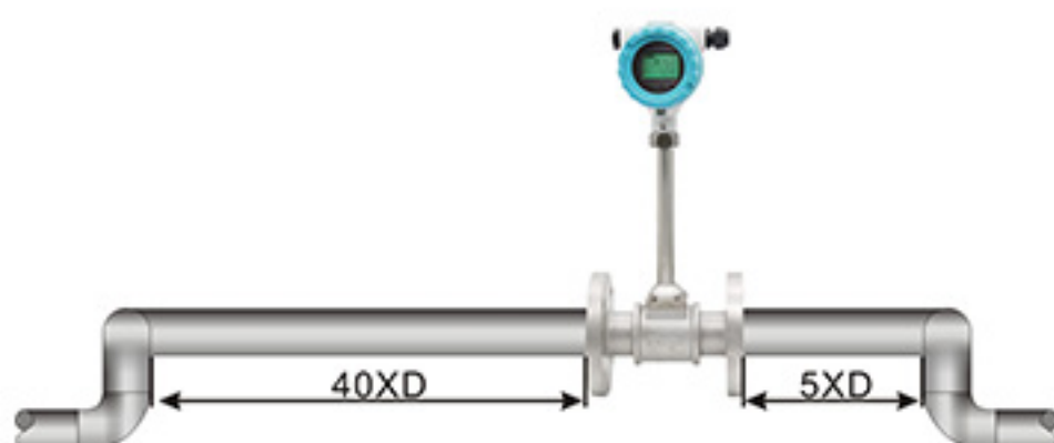
Two Square Bends At Different Plane
